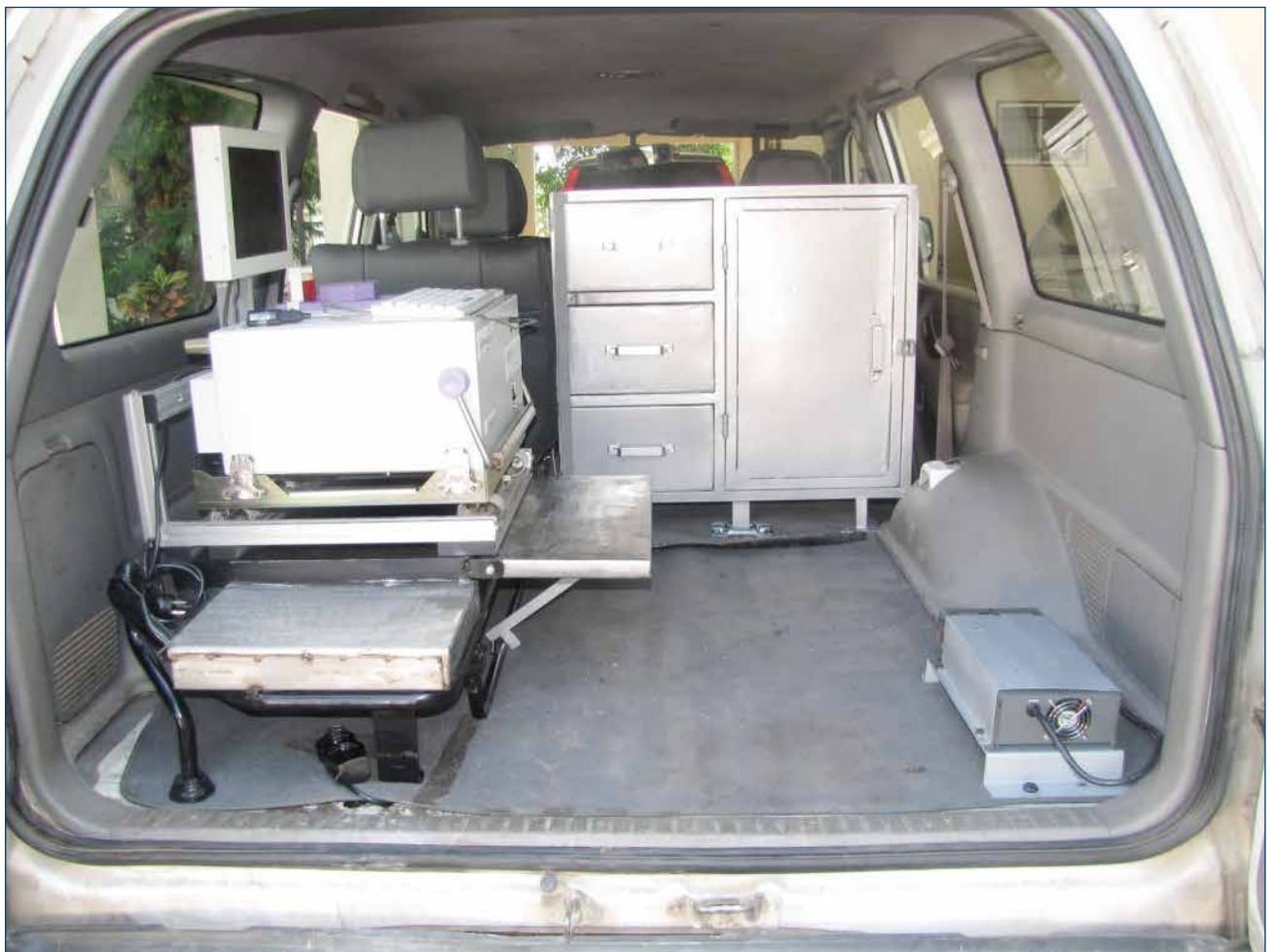
Figure 14: XRF Machine mounted inside a vehicle
